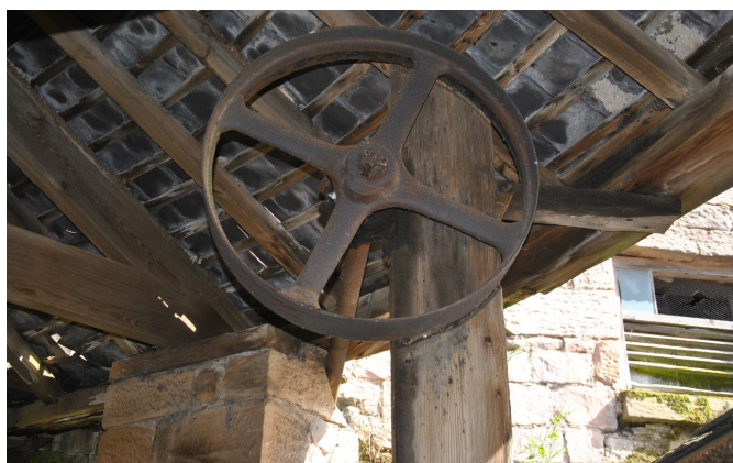
Inside the same Northumberland building, an iron drive wheel and shaft for the travelling steam engine that replaced the horses.
