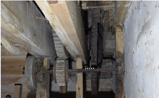
Inside a Northumberland barn, the wooden and iron gear wheels of a thresher are attached to the drive shaft entering through the wall at the right. The scale divisions are 10mm long.
