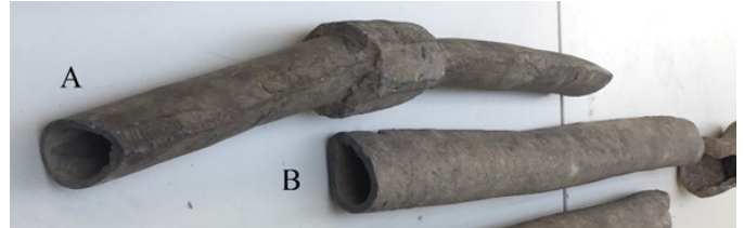
Fig 1: The two pipe sections tested, A with the box joint and B without. The pipes are made from a sheet of lead rolled up and soldered along the top.
